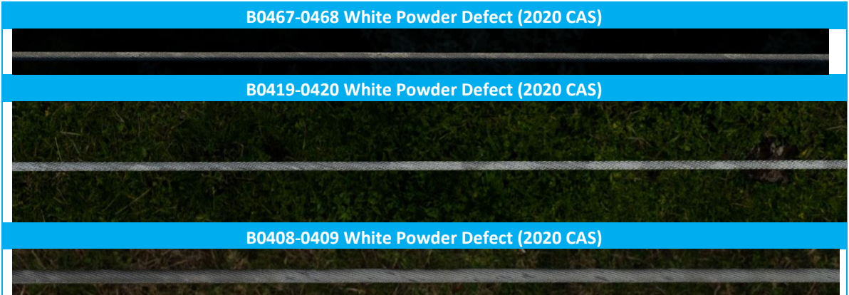
Figure 4. Examples of white powder defects found on the Stage 2 section of the OTA–WKM–B line
