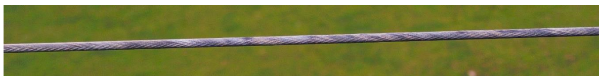
Figure 2. White powder defect in span A0475-0476 from 2016 helicopter inspection
