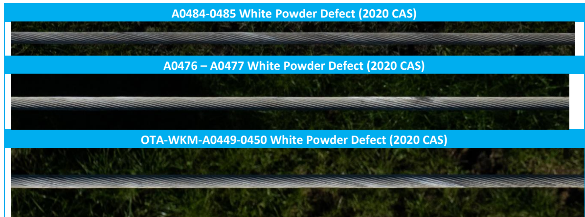
Figure 3. Example of white powder defects found on the Stage 2 section of the OTA–WKM–A line
